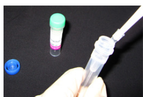
Step 5. Add 10 µl Reaction Buffer to NH 2 -Reactive Alkaline Phosphatase, and dissolve with pipetting. c)
