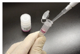
Step 3. Add 100 µl Washing Buffer to the Filtration Tube again.
